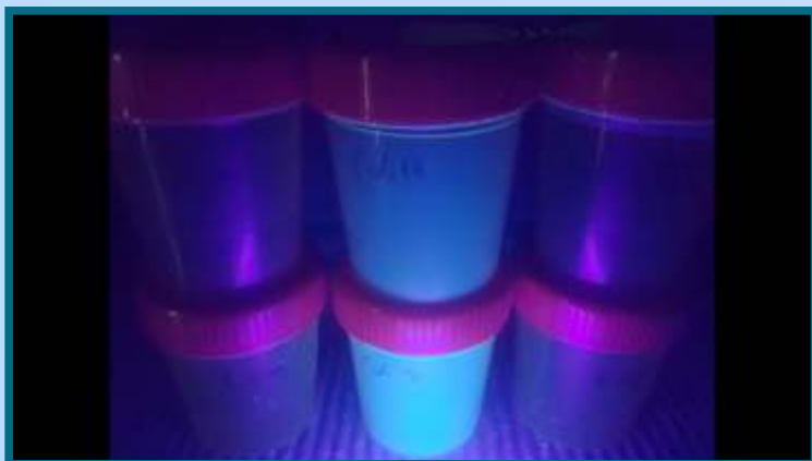
COLICULT-ISO 9308 , MUG reading in the dark under 366 nm: Center bottles, E.coli , fluorescent. Bottles from the sides, not E.coli , does not emit sky blue light.
