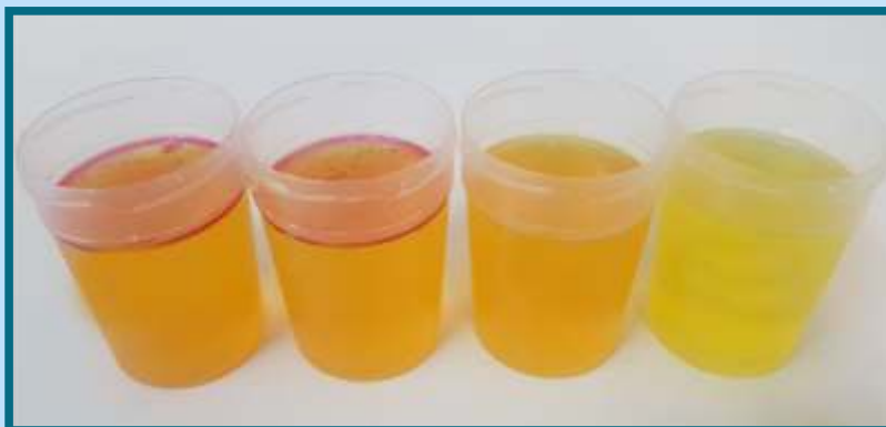
COLICULT-ISO 9308 , defined substrate (ONPG + turns from colorless to orange), indole (+ red ring) and fluorogenic (MUG + fluorescent). Bottles 1 and 2: E.coli . (ONPG +, Indole +, in the photo below, center, MUG +). Bottles 3 and 4: Non- E.coli coliform (ONPG + more or less intense, Indole -, in the photo below, on the sides, MUG -).
