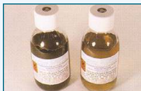
ENTEROCULT (BEA broth): Left + for fecal enterococci (black and opaque), right - (amber and transparent)
