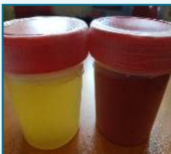
Chromogenic Vibrio cholerae P/A (chromogenic MPT broth): Left - (straw and clear), right + (red and opaque)
