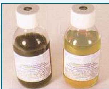
CLOSTRICULT (TSC broth): Left + for Clostridium perfringens (black and opaque), right - (straw and transparent)
