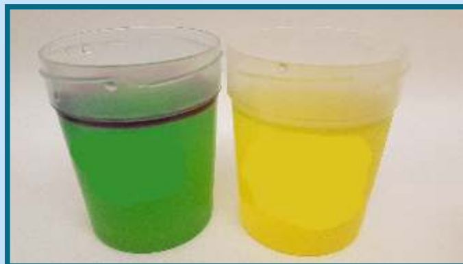
COLICULT-PLUS , defined substrate (ONPG + turns from colorless to yellow), indole (+ red ring) and chromogenic (MUGChrom + turns to green). Left E.coli (green, indole +) without having to read fluorescence. Right coliform (ONPG +) that is not E.coli (as it does not turn green and is indole-)
